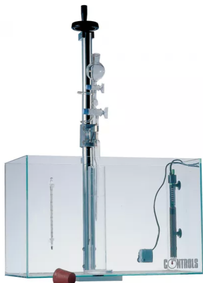
PARTICLE SIZE ANALYSIS SET: PIPETTE METHOD
